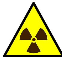
Figure 11 Basic radiation warning sign
