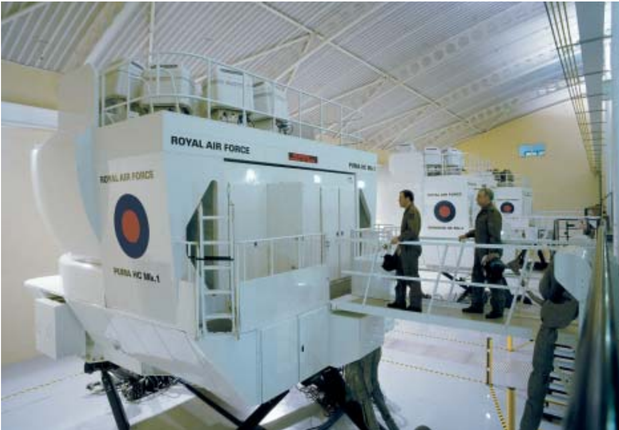
RAF pilots prepare to enter the Puma helicopter simulator at RAF Benson
