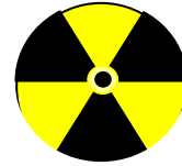
Figure 3 Marking for hazard grade radioactive valves. Colour of symbol: black on yellow background.
