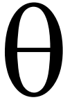
Figure 1 Theta marking for Class 1 radioactive valves. Colour of marking – black. (See Note.)
