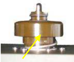
Wipe the inlet port under the rain cap assembly
