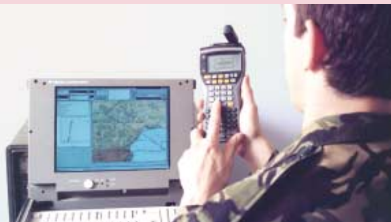
PRISM: A prototype computer based tool to track and log medical symptoms on the battlefield. Information tools on the battlefield, such as PRISM, will lead to improved support and effectiveness in operations and conflict situations.
