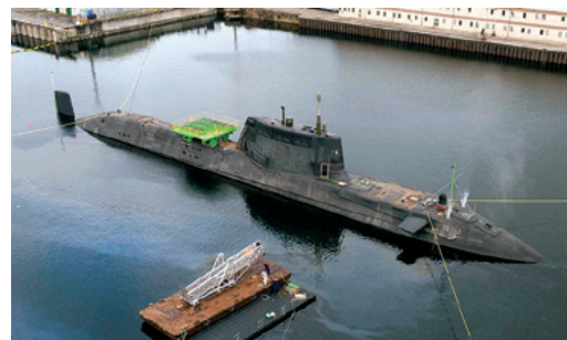
Astute class Submarine undergoes a trim test drive
