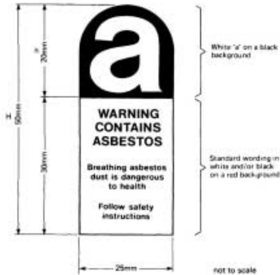
Figure 1 Asbestos Warning Label
