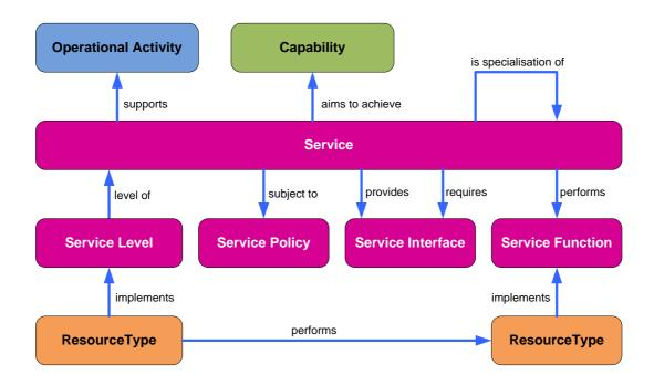
It should be noted that the SOVs are intended for specifying services for use in an SOA (i.e. loose-coupled, opaque service specifications). Services should <u>not</u> be used for simple interface management – SV-1 provides the concept of Resource Interface for this purpose.
