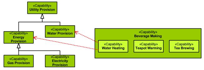
The dotted arrow points to the capability upon which another capability depends; ie the dotted line should read from tail to head: "depends on".
