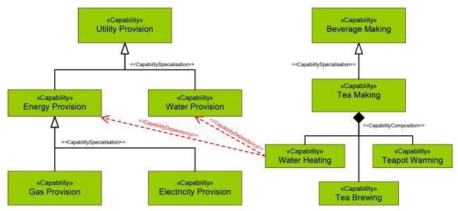
Example StV-4 (UML Aggregation Format – allows simpler combination of composition and specialisation)
