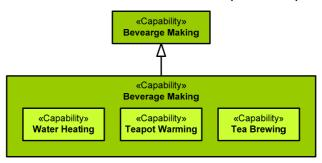
The ability to model capabilities as being components of other capabilities is part of the more general MODAF approach to modelling *dependencies* between capabilities.
