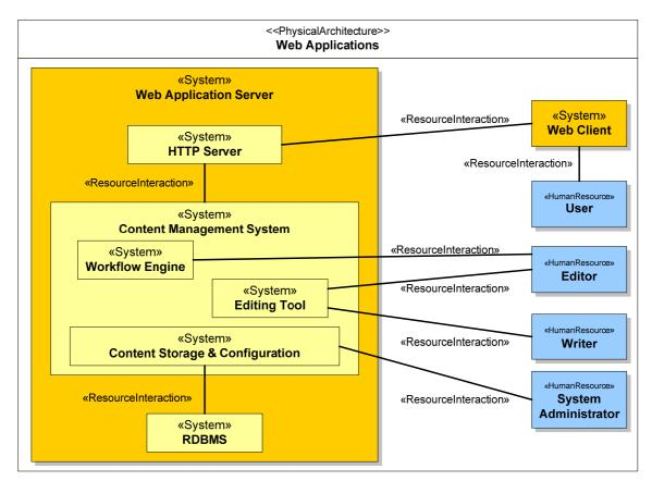
SV-1 Example (UML Composite Structure Model)
