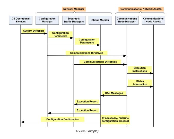
The figure on the following page shows an example OV-6c Product using a UML sequence diagram.
